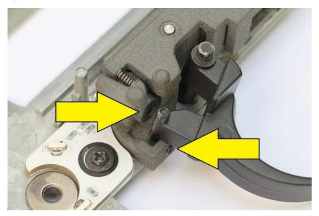
⚠ If the trigger will be putting pressure on the Clicker when at rest, the break force will be weaker!
