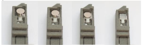
⚠ Note, that using these magnets with steel AK receivers will cause Clicker to become locked! However, this can be worked around by gluing a piece of non-ferromagnetic material to the top magnet, so that it does not stick to the receiver. Keep in mind, that with such solution the overtravel will be additionally limited.
